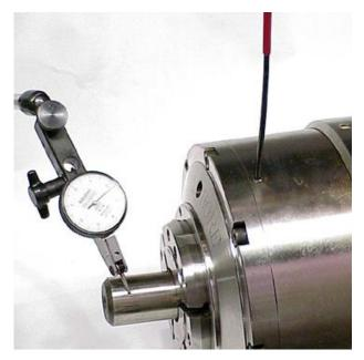
For high precision work, indicate the faceplate in using a piece of ground stock held in the collet pads. This procedure should be performed each time the collet or pads are replaced, if the accuracy requirements justify it.
