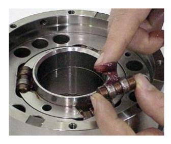
Install the roller and axle assemblies into the ramp. **LIGHTLY** grease the assembly to hold them in place for installation, and for lubrication after assembly.
