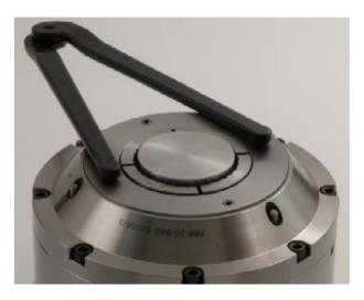
Clamping force or grip force is adjusted by screwing the adjusting nut in or out of the chuck. Grip force is increased by the clockwise rotation of the adjusting nut. Maximum clamping force is achieved when the indicator pins are flush with the counterbores in the faceplate. To reduce the grip force, rotate the collet counterclockwise until the desired grip is attained. With the force less than maximum, the indicator pins will sit at a position below flush with the counterbores.
