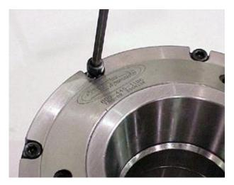
Install the faceplate/pusher combination on the chuck, making sure the indicator pins line up with the holes in the faceplate. Twist the faceplate/pusher combination while on the chuck so the bolt holes in the faceplate line up with the threaded holes in the chuck body.
