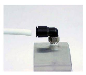
Connect air supply from the valve to the gland housing using the ½" airline supplied in the kit. The port in the gland housing is tapped 3/8 – 18 NPT. Cut off any excess airline and tie up loose or drooping line with wire ties.
