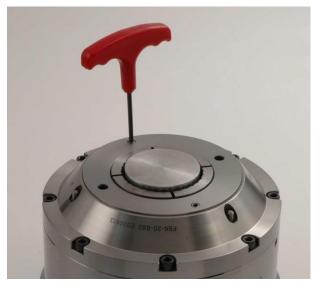
Adjust the clamping force by screwing the adjusting nut into the faceplate. This must be done with the chuck in the open position. Close the chuck to see if the indicator pins are flush with the counterbores in the faceplate. Reduced clamping force is achieved when the indicator pins are below flush, with the greatest clamp force having the indicator pins flush with the counterbores. Refer to the "**OPERATION**" portion of this manual for a further discussion on clamp force.
