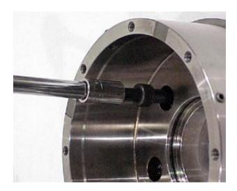
Mount the chuck body on the spindle, making sure the drive button in the spindle lines up with the counterbore in the back of the chuck body. Screw in the six bolts that hold the chuck body to the spindle. Alternate between opposite bolts while tightening. Put the machine in the spindle lock if equipped, or lowest gear to prevent the spindle from rotating. Two of the faceplate mount bolts can be screwed into the face of the chuck, and a bar can be placed between these for leverage.
